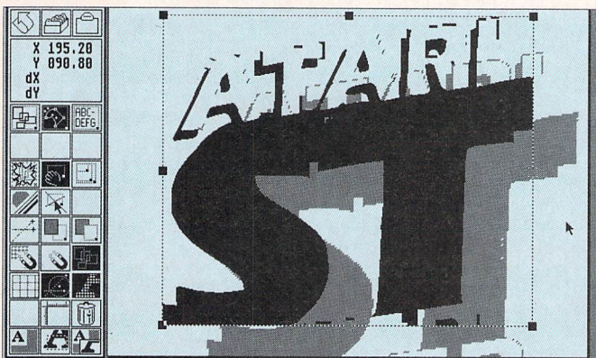
Here the vectorised ST User logo has been offset against the scanned pixel version. Most autotraced images require a good deal of further editing
