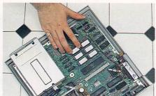
Locate the old TOS chips in your machine, and make a note of where they go. All the chips are numbered in order, and should be carefully removed and replaced by their 1.4 equivalent. Make sure the small notches on the chips match up with those printed on the motherboard. Chips are sensitive to static, so handle
