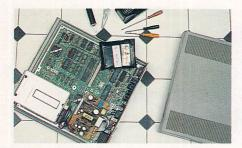
Disconnect the ST from the mains and unplug any peripherals such as printers. Then remove the upper casing from your ST - be careful of the wire attached to the underside of the case. Carefully untwist the tabs holding the metal shielding in place and remove that as well
