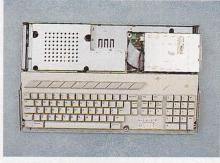
3. BELOW: Disconnect the leads which connect to the back of the drive
