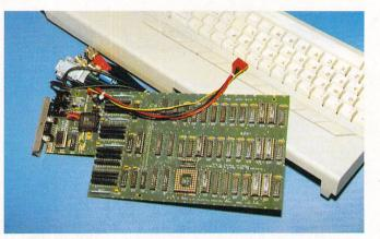
The ISAC colour board for Mega STs. Provides s a full A3 colour screen when hooked up to a suitable Multisync monitor
