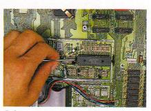
Before you can use the ST Video Box you must strip down your computer to the bare circuit board and prise out the shifter chip...
