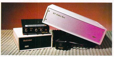
The ST Video Box from IMR is massive in comparison to the tiny GST 40E from TCT. The Multidat unit from IMR is a handy video splitter that takes the ST's monitor output and pipes it down four separate cables to four different monitors. Great for shop windows and shows
