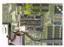
... and slot this tiny PCB into the socket. The shifter chip is then plugged into the socket on the new PCB
