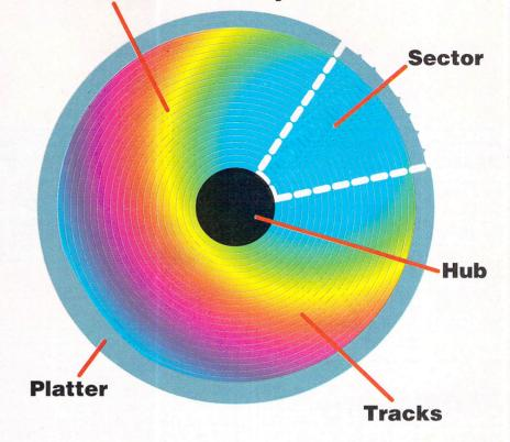
over it telling you not to think about removing the case Why? Because opening the case lets in air. Platters are kept in a vacuum which is totally dust free, air has all sorts of junk floating around in it. A hard drive's heads don't actually touch the surface of the platters but they are positioned very close to the surface, floating 20 millionth of an inch away from the platter's surface. A human hair is about a 100 times thicker! Even smoke particles would wreak havoc at these tolerances.
