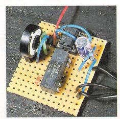
This is the upper, component side of the Slowmo circuit. Pay particular attention to the orientation of the chips and capacitor. Notice also that although in the text it is recommended that both chips are placed in sockets, here the macho solder master has decided to do without the relay - what bravery!
