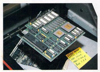
RAM upgrades for ordinary STs could soon be as easy as plugging in one board like this prototype from GE-Soft
