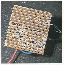
Soldering together such small strips can pose problems for the beginner. Some tips: try to use as little solder as possible to avoid a mess and/or a potential short-circuit. Try to minimise the amount of time the hot iron is actually in contact with the components. If you bake them too long, they'll break.
