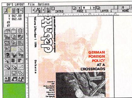
The cover design was a scanned image used as a background tint, with a section cut out and re-inserted in its original (though slightly retouched) appearance. This sort of trick is very effective as the full scan would have distracted from the text and logo
