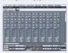
The Midi Mixer lets you automate the mixing process. This shows the Filter section which offers three-band EQ, pan and volume control
