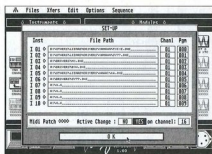
You can make up to ten instrument drivers load automatically when the program boots
