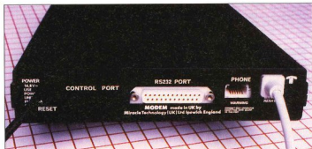
The connections on a typical modem. Note that you'll need a new-style phone socket and lead to get connected
