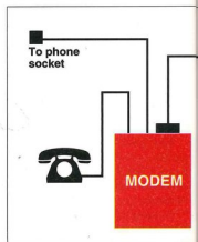
Connecting a modem into your ST setup. Note that as the telephone plugs "through" the modem, it will be unusable when the modem is in operation
