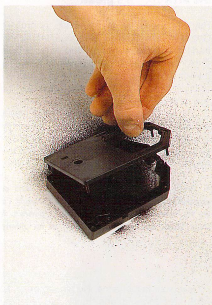
Replace the cartridge's lid. Remember to leave the ribbon for 24 hours before using it
