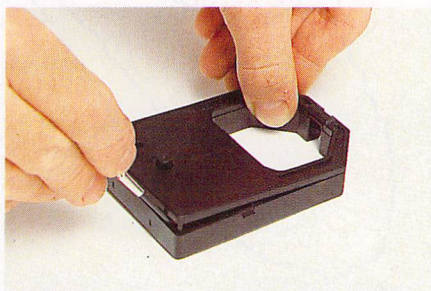
Carefully remove the cartridge's lid. A small screwdriver should do the trick
