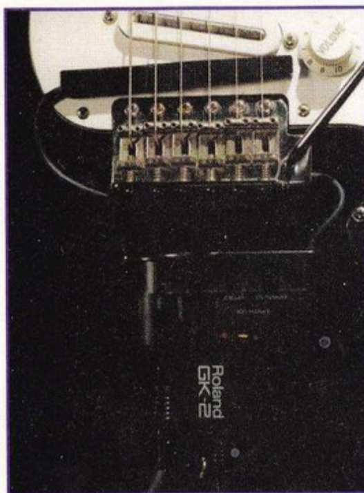
The GK2a unit can be positioned anywhere on the body of your guitar. The volume control is a MIDI controller that governs the overall volume of the sound you are playing.
