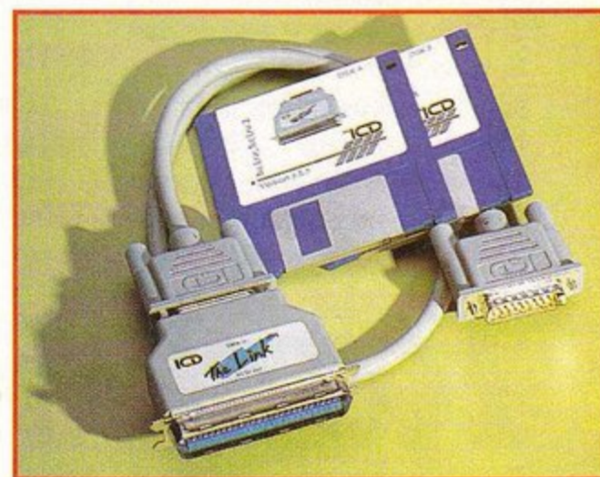
You'll need a DMA-SCSI interface (such as ICD's The Link) to connect the EZ Drive to your ST. These cost around £50.
