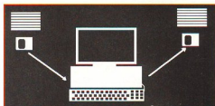
Data from drive A is loaded into your computer in 32K blocks, using BLOAD. It can then be saved on to drive B, using BSAVE.
