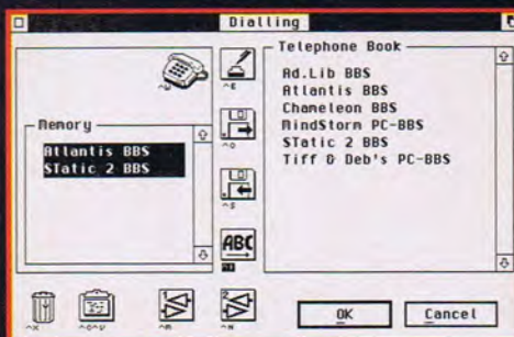
■ The Dial screen stores your BBS numbers. Double-clicking a name on the right dials it, and multiple numbers can be dropped into the memory store on the left, so you can dial a selection one after another.
