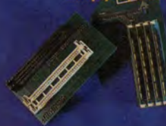
■ FalconWing: if you want to upgrade from 4MBytes to 16MBytes later on you simply replace the SIMMs.
