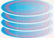
■ The actual disks, or platters, in a hard drive are parallel to one another. There are separate heads for each side of each platter which move in and out from the edge of the disk towards the centre in exactly the same way as in a floppy drive.
