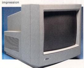
of a final colour. Get up close to the screen and you find that each pixel is, in fact, made from a collection of dots coloured red, green and blue – the different intensities of the colours give you the final colour. It's an additive colour system; if you have maximum intensities of
