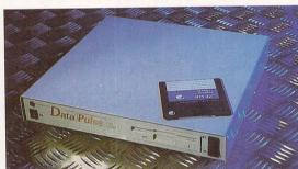
normal drive. We used the floptical drive from Ladbroke constantly for over a week, with no problems saving and loading data. The manufacturers of the disks claim it is impossible to corrupt data on the disks, and we certainly found no reason to dispute this. Data transfer rates to and from the disk are slower than a hard drive at around 162.5K/s (1.5Mbit/s)
