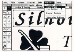
■ Using the Clip tool, an adjustable Clipbox is defined to enclose the section of the image you want to work on - you can choose the size of it.
