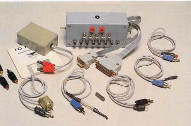
• The Switchsoft I/O Port, with the Sensor and Control Experimenter's Kit. The Kit costs £27.95 and comes with six projects, covering LEDs, motor control, reed switch and magnet, light control, tilt sensor and switching.
