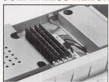
Upgrade the memory of your ST quickly and easily with our new, fully software compatible RAM upgrade board. Designed for pre-STE machines, the unit accepts SIMMS slot-in memory modules, making RAM fitting simplicity itself. No electronics knowledge needed! Available with or without RAM modules. Allows upgrade in stages of 1Mb, 2 / 2.5Mb and 4Mb, as and when necessary. Straightforward installation full, comprehensive instructions provided.
