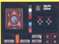
■ EDITING SPRITES summons an editor box with a blow-up view of a 24x24 sprite. Eight colours can be used from a palette of 512
