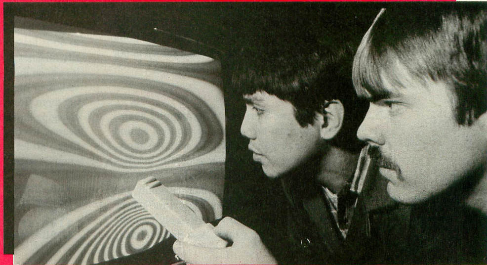
Workers test a TV picture tube for color quality.
