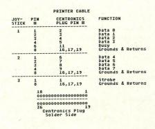
You can use IDC plugs and ribbon cables, but I found the joystick replacement cables as easy as any to use. When done, plug the 36-pin plug into your printer and the joystick cables into their proper outlets on your Zucchini. Run the following program to test the cable:
