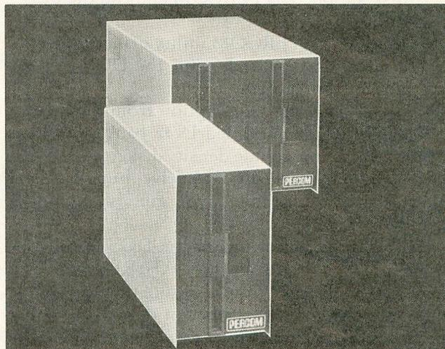
The PERCOM drive controller will detect whether a disk is single density or double density during the boot process and switch to the correct mode of operation, making it suitable for use in an ATARI system. Even when it is the only drive in the system, single density disks will cause the drive to operate in single density mode.
