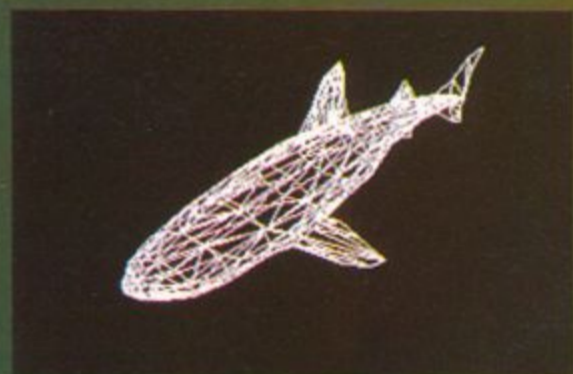
Sculpt4D enables you to construct objects from a set of polygons - there are over 200 in this image.
