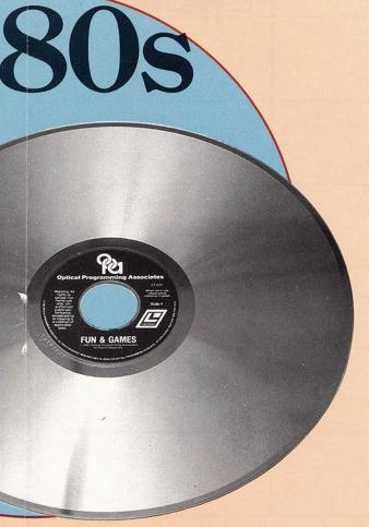
laser videodisc is a flat, round piece of plastic that is about the size of a 33 1/3 RPM record. It can store pictures that show motion, much like a video cassette tape stores movies. Like a video tape, a laser videodisc can also store sound and written text. A single disc can hold all the words contained in 170,000 books. A laser videodisc runs on a laser videodisc player.
