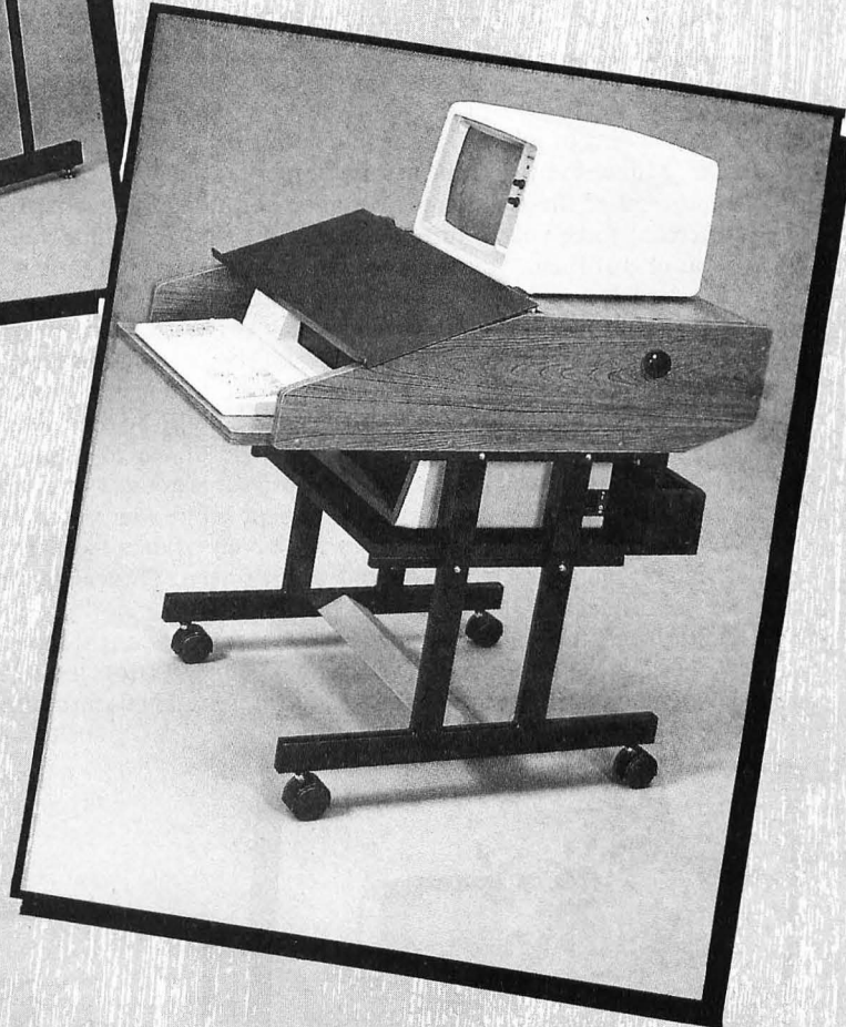
Photo 3: In the Data-Leggett 3028C, HSP paid considerable attention to the details of good human engineering. An unusual feature is the slanted document holder between the keyboard and the screen. The platform for the monitor is tiltable, for avoiding glare. HSP also places the keyboard at a somewhat lower height (23 1/4 to 25 1/4 inches) than the commonly-accepted 27 inches, preferring a steeper angle of the forearm to the floor (0 to 15 degrees).
