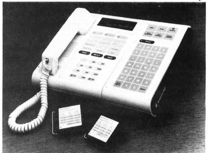
American Bell's first effort toward the futurephone is their Genesis system. The plug-in cartridges add various optional features, such as call forwarding.
