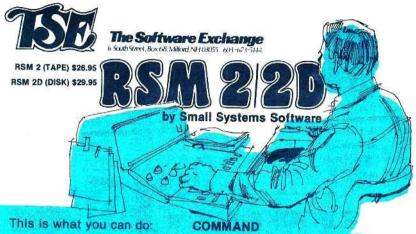
A - ASCII DUMP: B - BINARY ARITHMETIC: C - CHECK TAPE: D - HEX DUMP: E - EDIT: Enter, examine, or modify memory in hex code F-FIND 1 BYTE: G - GOTO: Go to and execute program at specified address H - HUNT 2 BYTES: I-INITIALIZE/INPUT: K - KEYBOARD ECHO: L - LOAD AND GO: M - MOVE: O - OUTPUT: Q - CHECKSUM: R - READ TAPE: S - SYMBOLIC DUMP: T. TEST MEMORY: U - USER: V - VERIFY MEMORY: W - WRITE TAPE:
