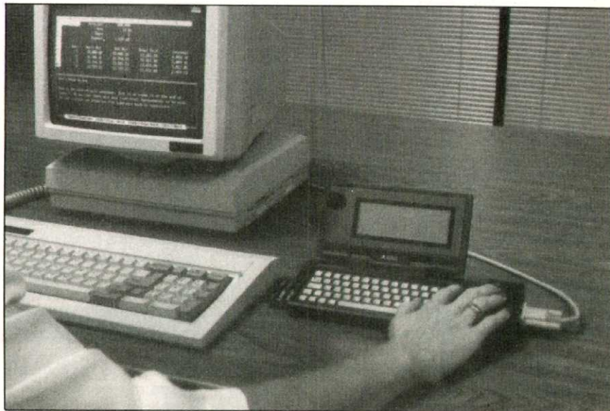
Smart parallel interface lets the Portfolio transfer files to and from a desktop PC.
