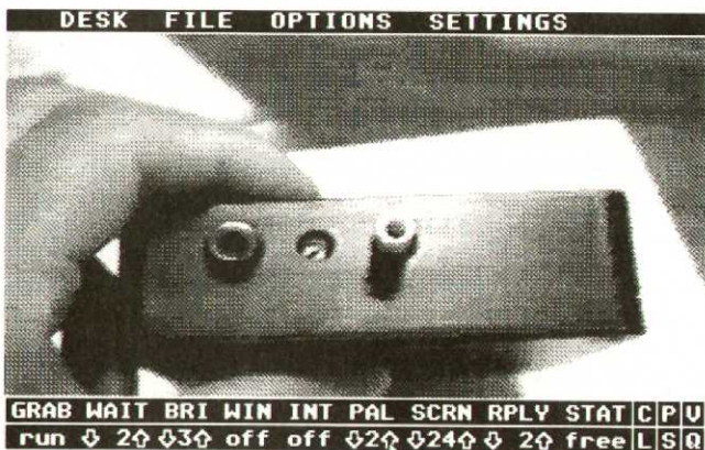
Figure 2. Front view of the Vidi-ST cartridge, showing the contrast, brightness, and scanning frequency controls.
