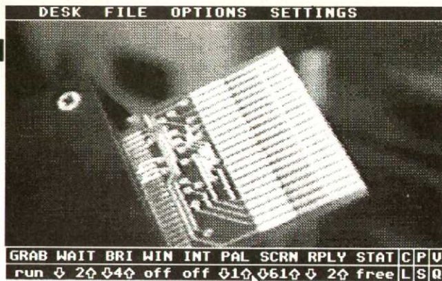
Figure 1. Closeup view of the Vidi-ST cartridge, showing the edge connector. The Vidi-ST main menu is overlaid on the image.
