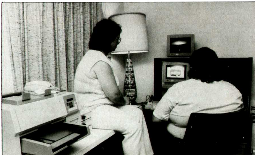
The Waldrons' desktop publishing system includes an Atari ST, a 20Mb Megafloppy hard disk, an Omnilaser 2103 printer, and an ST Scan image scanner.
