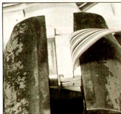
Photo 3. Squeeze only hard enough to close the connector.
