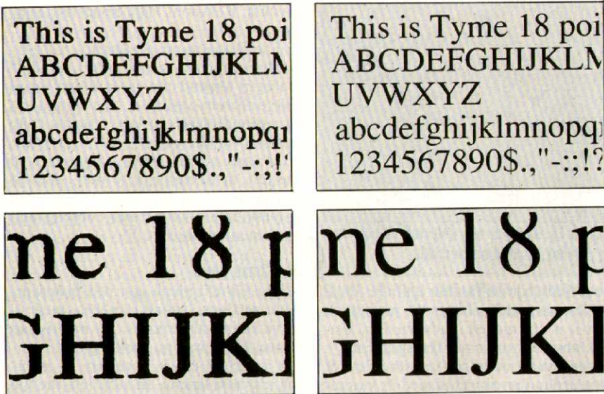
Figure 17. Comparison of laser printed type with output from a Linotron typesetter at 2400 dpi using the ability of PageStream to save files in Postscript format. Samples are shown actual size and magnified 300%.
