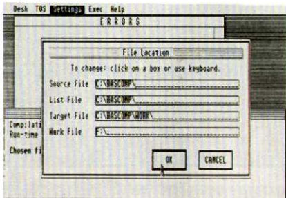
The shell permits you to configure a programming environment with separate source, list, and object pathnames.
