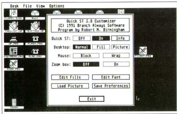
**FIGURE 1.** QST3CUST.ACC, Quick ST's "customizer" accessory, gives full control of the program's many options.
