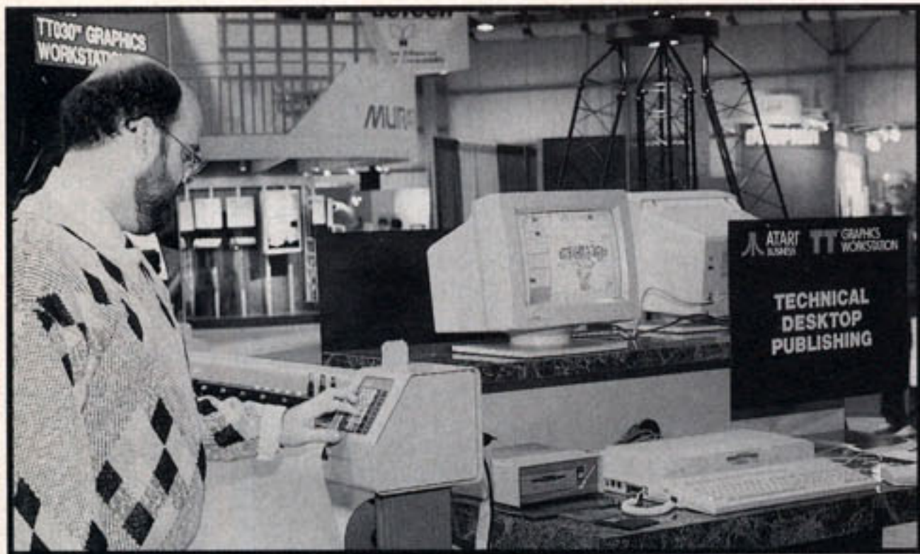
Mario Perdue, of CADRE, Inc., demonstrating DynaCADD (ISD Marketing); a powerful tool for ST-based Computer-Aided Design and Drafting. The TT030 is driving a Houston Instruments plotter.
