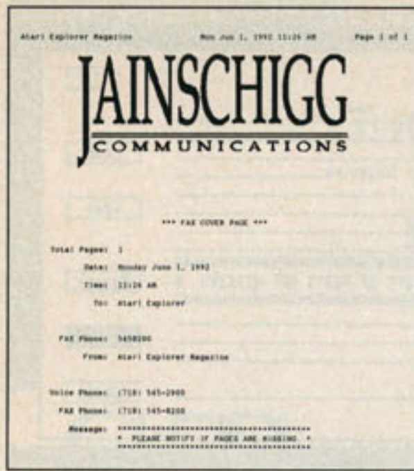
FIGURE 3. Attractive output at the destination is just one of the advantages of STraight FAX' all-digital approach. Documents can be converted directly to fax "images," free of the distortion that can be introduced by optical scanning.
