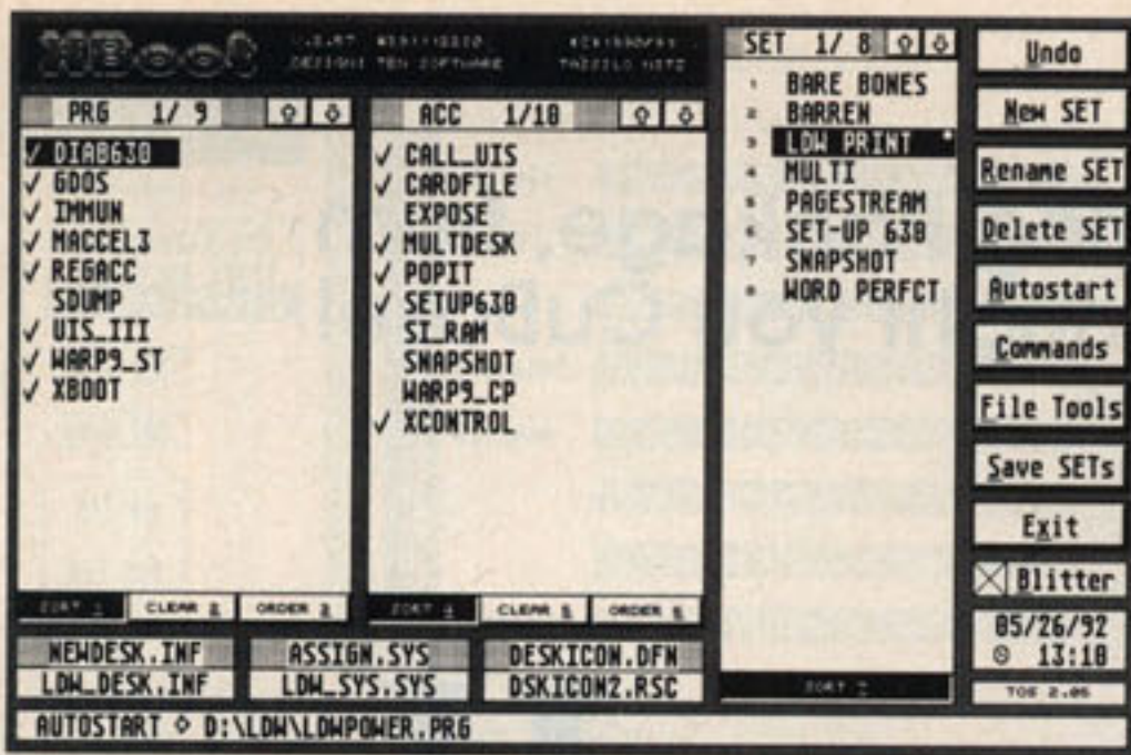
FIGURE 1. XBoot's Boot Manager lets you create working "sets" of AUTO folder and programs and .ACCs
