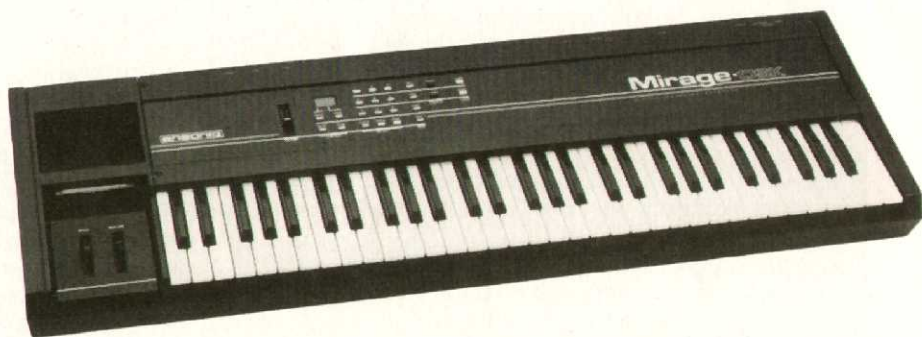
The Ensoniq Mirage. Note the almost-full-size (61-note) keyboard and disk drive slot.
