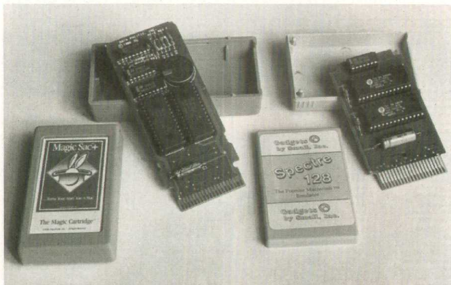
Figure 1. Spectre 128 (right) is much smaller than the older Magic Sac, but doesn't have built-in clock.
