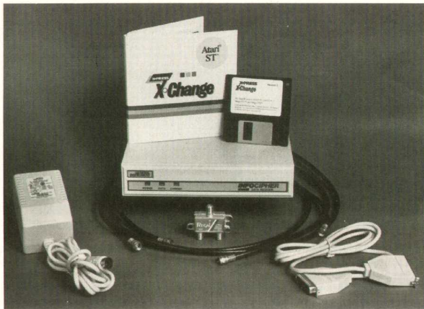
Figure 1. Hardware and software that comes with the X*Press startup package. Note decoder and Y cable splitter.
