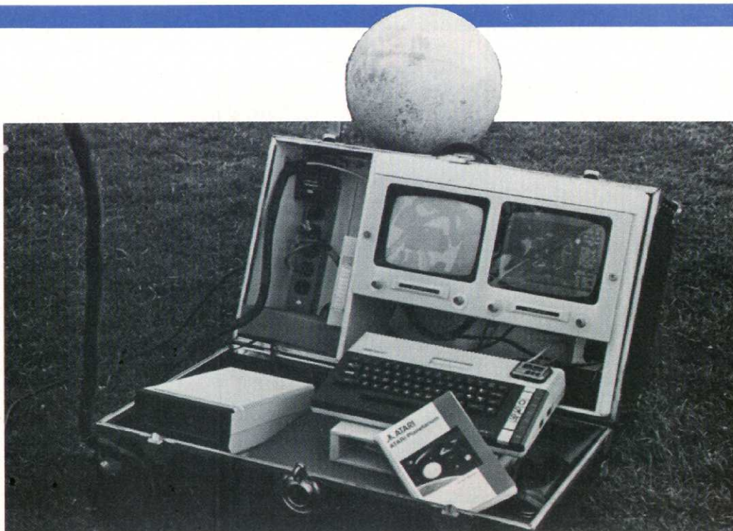
The author's portable planetarium features an image of the moon on-screen at left and a red-filtered computer display of the night sky at right. The moon globe atop the trunk aids in instruction.
