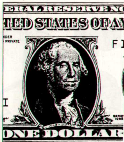
Figure 6. Portion of dollar bill scanned at 300 dpi and printed at the same density on a laser printer.
