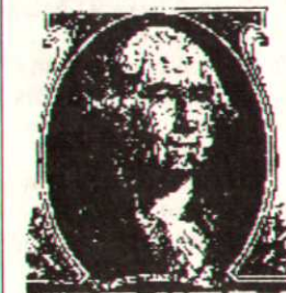
Figure 3. Portion of a dollar bill scanned at four densities (300 dpi to 75 dpi) and printed at 180 dpi on a 24-pin dot matrix printer.
