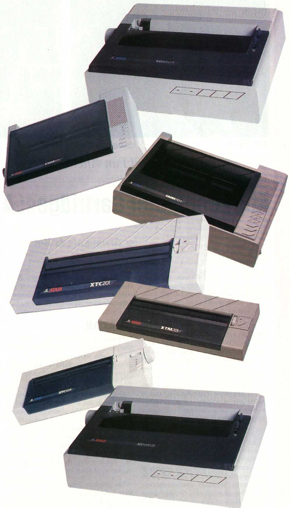
Printers that run the gamut—letter quality daisy wheel, high speed dot matrix, and low-priced color and monochrome thermal transfer dot matrix.
