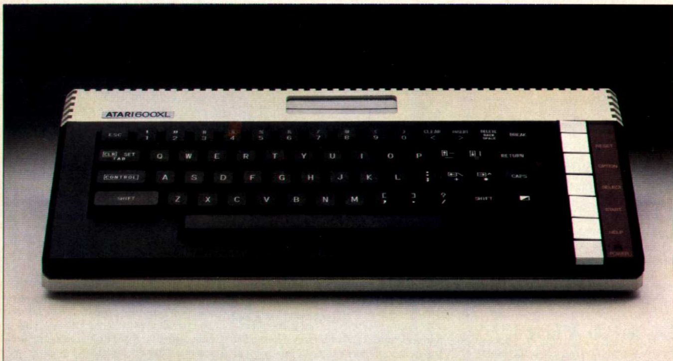
Atari 600XL. Built-in BASIC and new parallel interface port on back.
