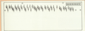
Figure 11: Layout showing the position of the slides on the reverse of the PCB
