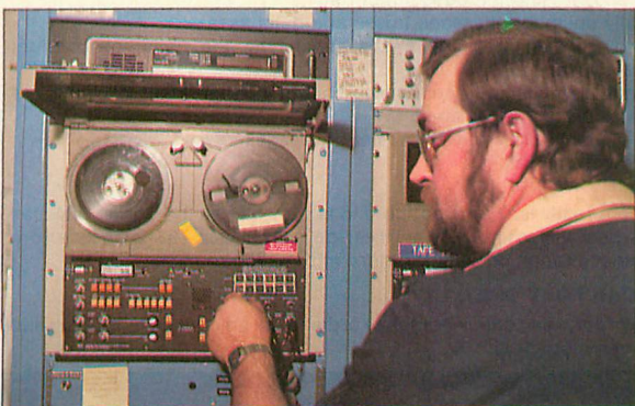
Ready to broadcast: Satellite photo data is translated into audio tones.
