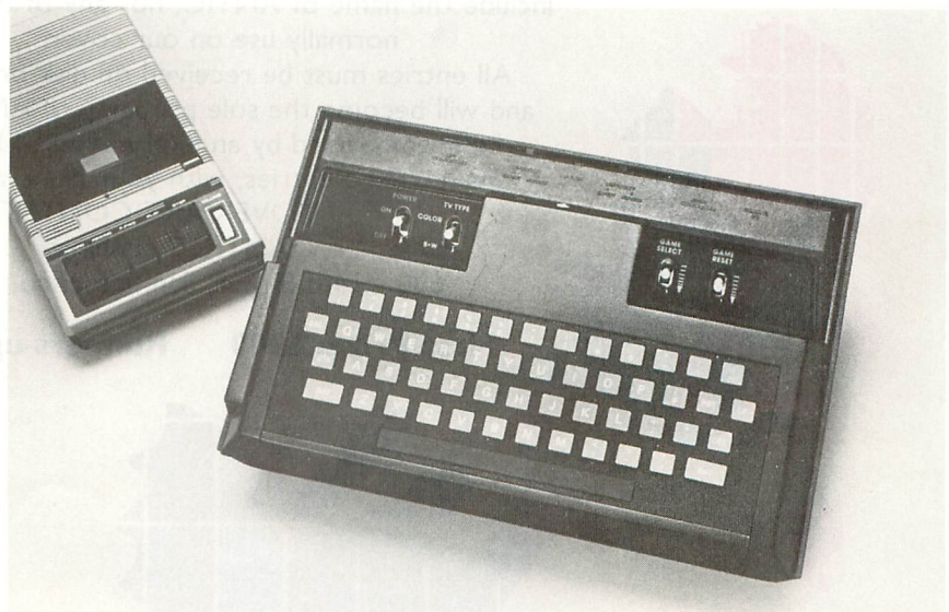
My First Computer, an easily-installed, plug-in keyboard converts the Atari 2600 video game player into a programmable 8K computer. Lower photo shows unit installed on VCS. A standard cassette tape player can be used for external memory.
