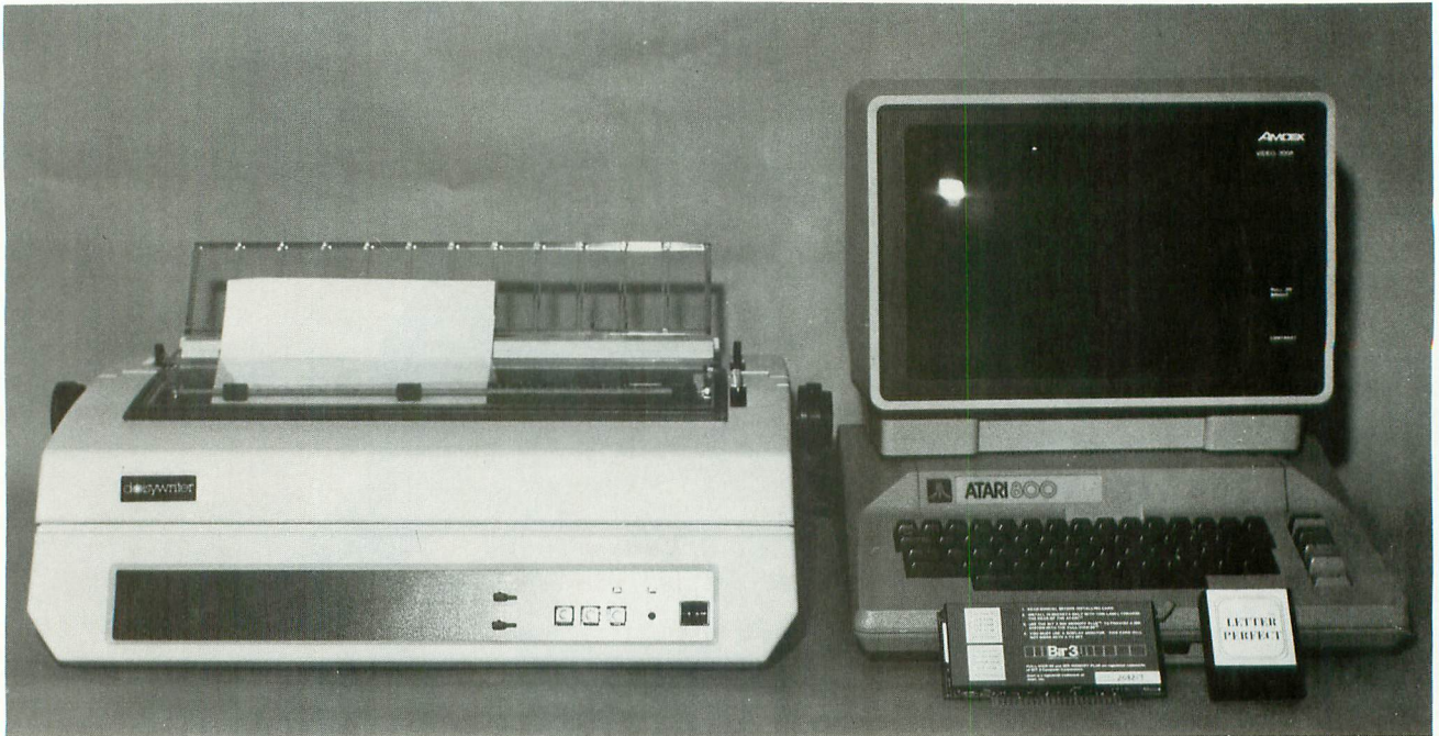
MODEL WORD PROCESSING STATION — The ATARI 800 with 48K RAM, the Full View 80-Column Board by Bit3, LJK's "Letter Perfect" Word-Processing Program (80-column cartridge version), Amber Screen Monitor by Amdek, and the Daisywriter letter-quality printer from Computers International. Percom double-density disk drives were also used, although in single-density mode.
