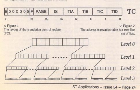
The MMU checks that the field sizes and the page size are consistent, and gives an error during configuration if not. To keep it happy, the total sizes of fields A to D, plus the number of bits of address space determined by the page size must come to exactly 32 (the size of an address). The field sizes determine the number of entries in each table: if field B is six bits wide, then there will be 64 entries in each level 1 table.
