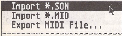
Fig. 5: The File menu allows you to import two very important file types - MIDI files from many many sources and .SON files from Notator SL V3.x. SL loaded files produce up to 4 Logic 'folders' (similar in concept to GEMDOS folders) longways across the screen. These can be unpacked into individual sequences if you need to continue editing. If your SON files have tempo changes, however, you need to create a sync reference first or you are back to fixed tempo throughout.
