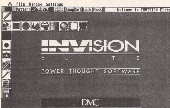
The opening screen from Invision showing the Pop-out icon bar, the Status line across the top of the screen below the menu bar, and the desktop icons. Everything on the Desktop can be positioned as desired.
