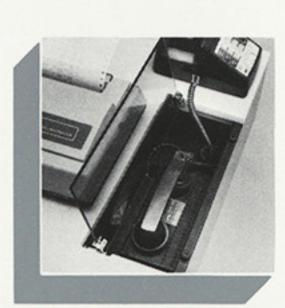
have a Data Recorder and the optional Modem. Voice contact is first established, then the Modem is engaged and all data is collected.
