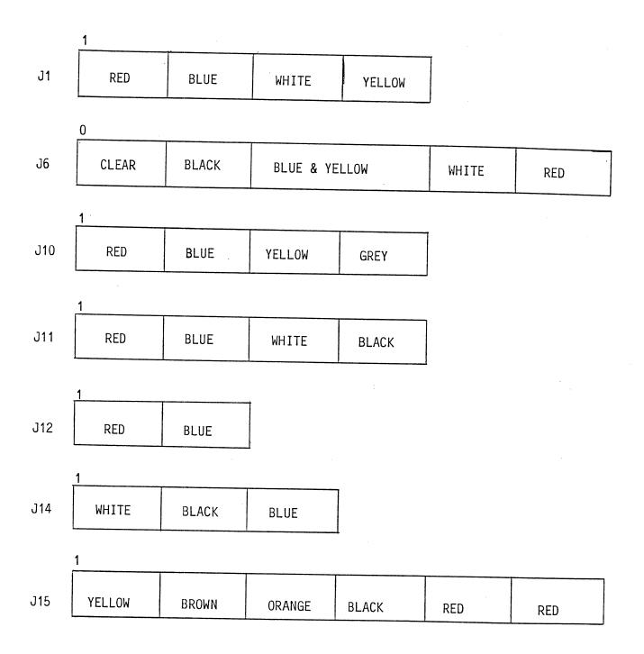
Plug Connections of 1050 Drive Mechanism
