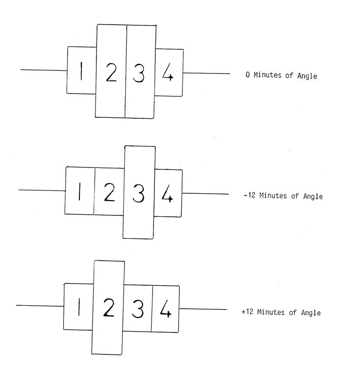
Head Azimuth Waveform
