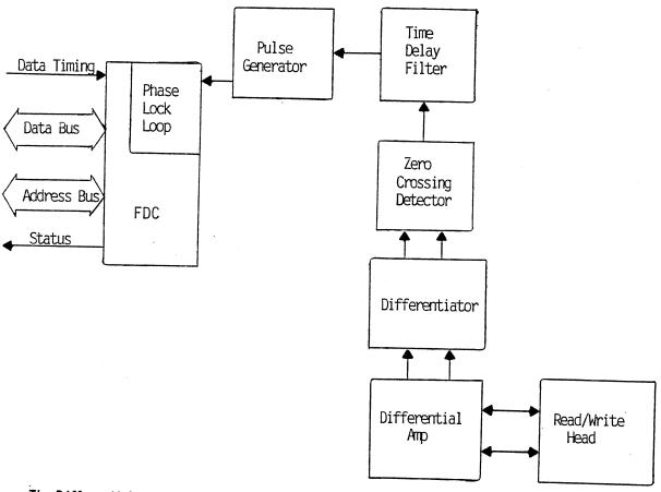
The Differential Amp provides initial amplification of Read/Write head signals.
