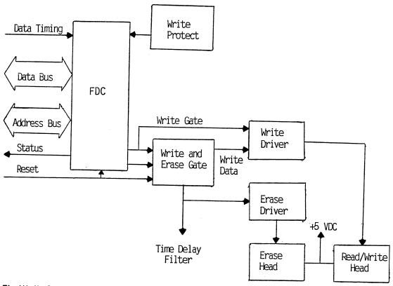
The Write Driver enables Write functions and limits the Write currents.
