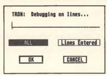
The Tron option displays the program's line number in the Command Window as each program line is executed.
