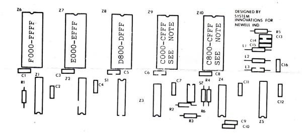
NOTE: Socket Z9 can be addressed as  ${\tt C000-C7FF}$  or  ${\tt C000-CFFF}$  depending on the setting of S2
